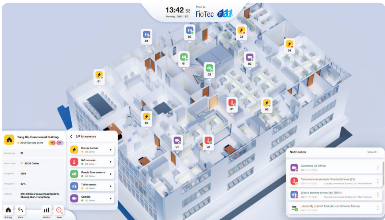
A customised and 3D BIM-enabled dashboard showing real time status of all IoT sensors developed by FioTec
